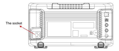
Figure 2-1 Connect power line
