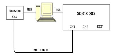
Figure 4-2 Clock Accuracy adjusting environment
