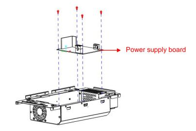
Figure 5-6 Removing the power supply board
