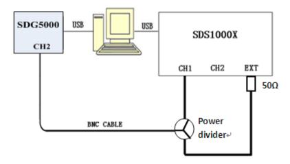
Picture 3-3 Connecting test instruments for Ext Trigger Delay
