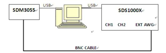
Picture 3-6 Connecting test instruments for AWG Offset Accuracy
