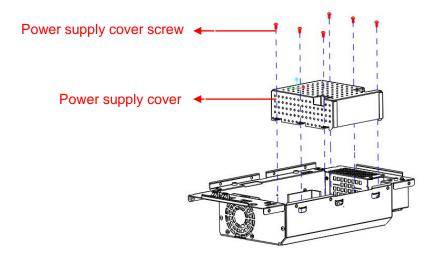
Figure 5-5 Removing the power supply cover
