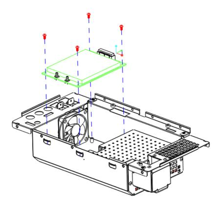
Figure 5-5 Removing the rear metal cover
