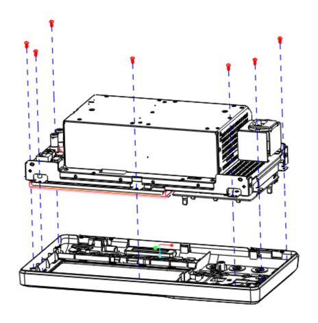
Figure 5-3 Removing the front panel
