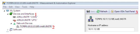
5. Click "Open VISA Test Panel" option button, which then displays the following interface. Then click "Input/Output" option button and click "Query" option button; you will see the Read operation information.
