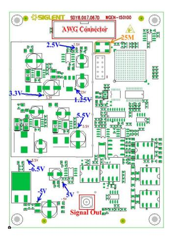
Figure 6-2 AWG board module
