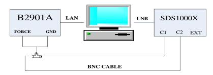
Picture 3-1 Connecting test instruments for DCG\Offset
