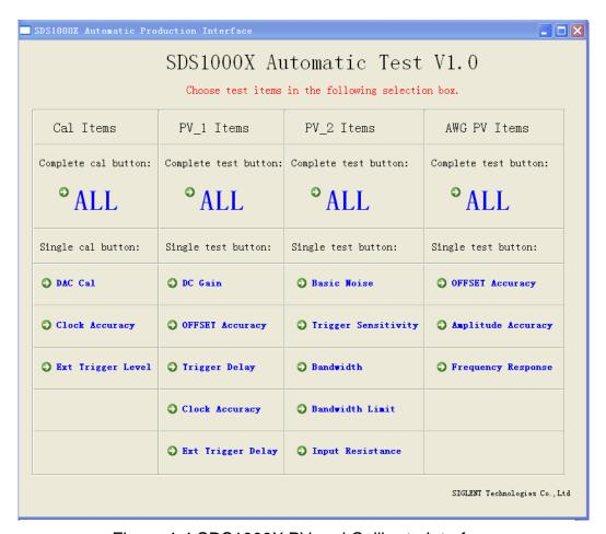
Figure 4-4 SDS1000X PV and Calibrate Interface
