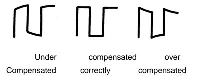
5. If the waveform does not show as "compensated correctly", use a nonmetallic driver to adjust the low-frequency compensation adjustment hole on the probe until the waveform displays correctly.
