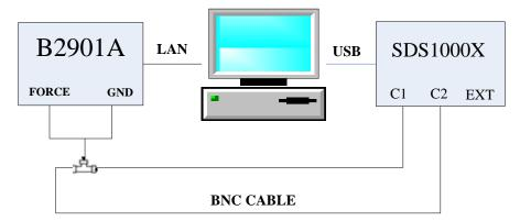
Figure 4-1 DAC adjusting environment
