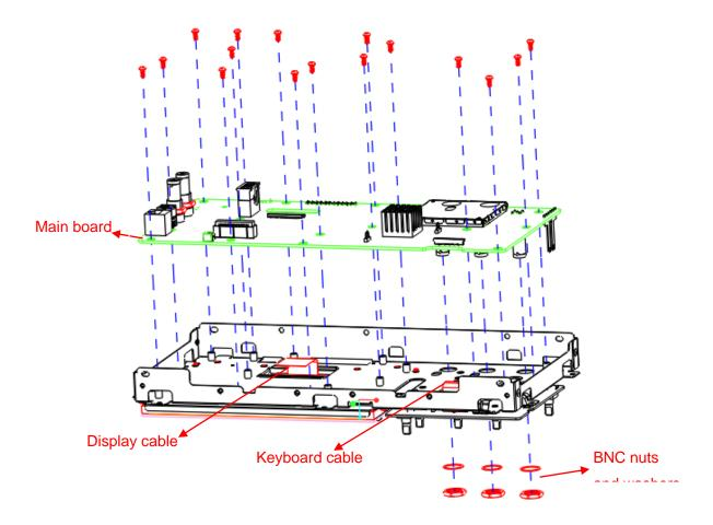
Figure 5-8 Removing the main board
