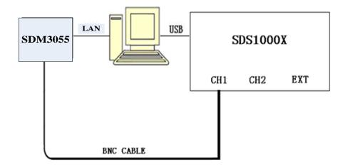
Picture 3-5 Connecting test instruments for Input Impedance
