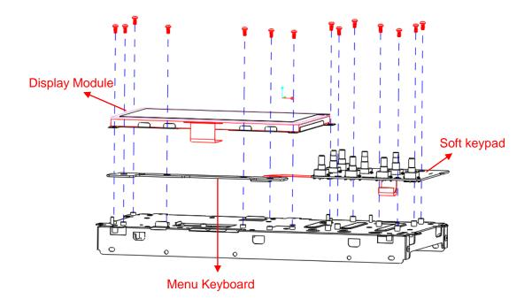
Figure 5-10 Removing the keypad and display Module
