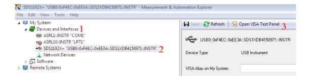
4. Click "Open VISA Test Panel" option button, and then the following Interface will appear. Next, click the "Input/Output" option button and click the "Query" option button in order to view the Read operation information.
