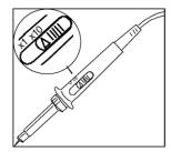
Figure 2-2 Set the attenuation switch
