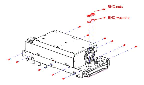
Figure 5-4 Removing the rear metal cover
