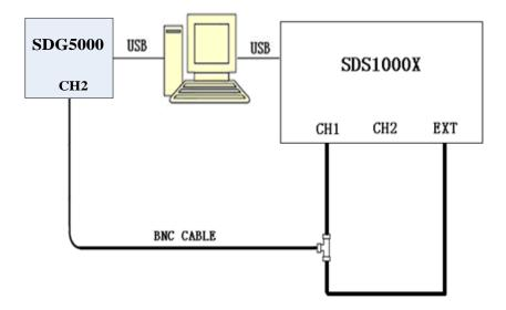
Figure 4-3 EXT Trigger Level adjusting environment
