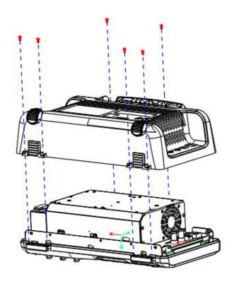
Figure 5-2 Removing the rear panel
