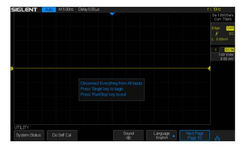
Figure 2-3 Calibration interface
