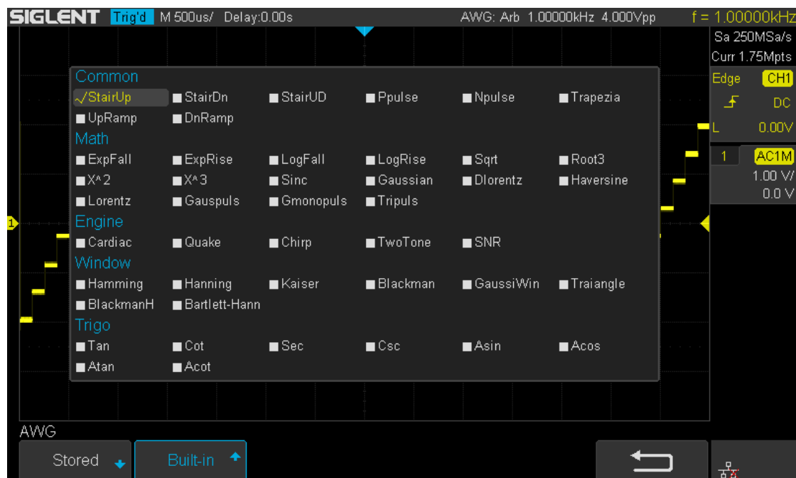
Figure 117 Built-in Arb Interface
