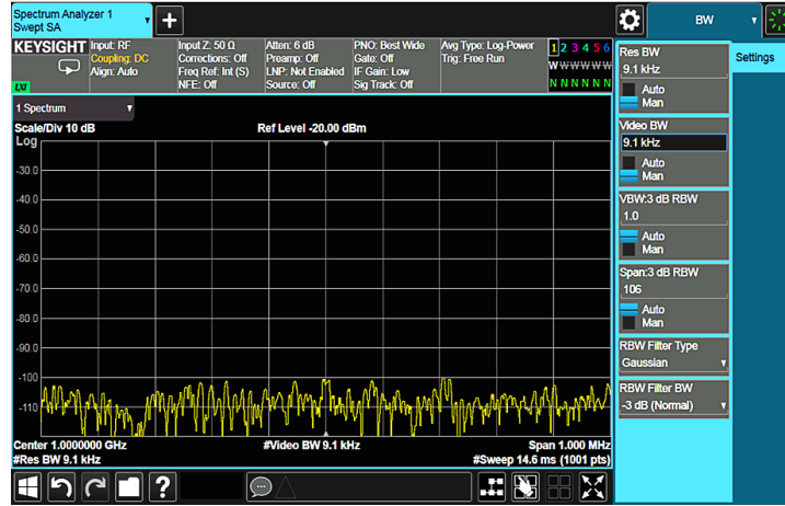
Figure 2-27. Spectrum analyzers display signal plus noise
