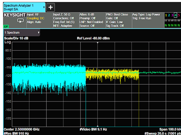
Figure 2-29. Smoothing effect of VBW-to-RBW ratios of 3:1, 1:10, and 1:100
