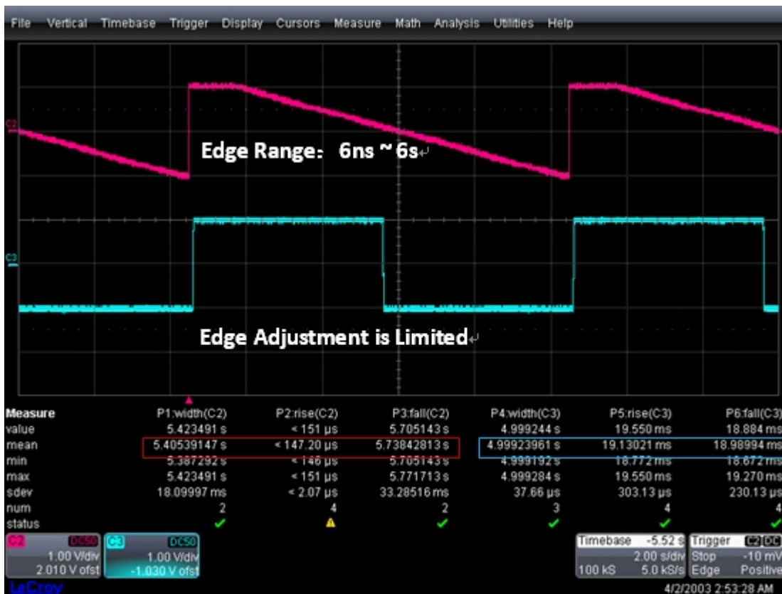
P3 Comparison of edge adjustment of low frequency 0.1Hz pulse signal
