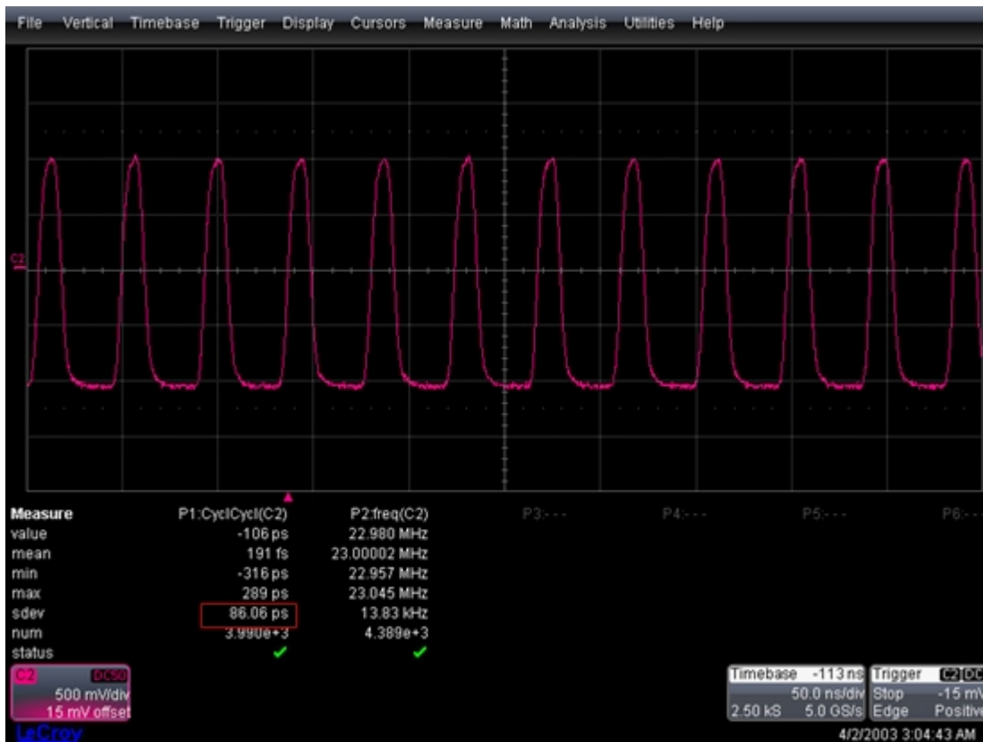
P4 EasyPulse waveform with low jitter
