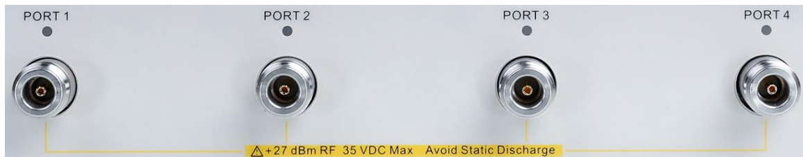
Figure 5-3 Front panel RF connectors (4-port-VNA)
